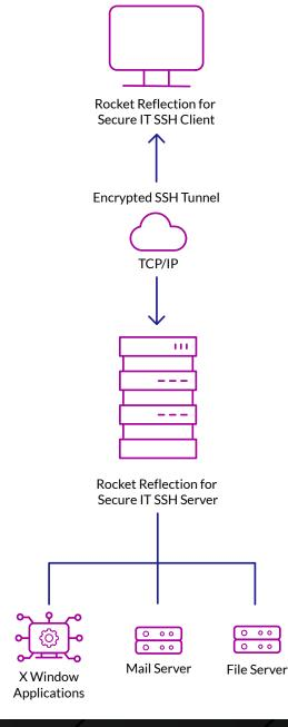
**Fig 1.** Together, the SSH client and server form a secure "tunnel" through which all communications travel.
