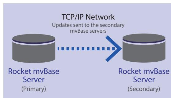
With FFR, downtime can be virtually eliminated; the only possible data loss would be to any updates that were not successfully received by the secondary mvBase server at the time of the system failure.
