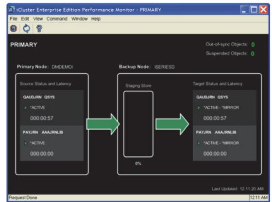
The graphical performance monitor shows you the source journals and target journals. A simple green arrow indicates that the replication is active for both the send and apply. A gas gauge shows you when reorgs or refreshes are in process.
